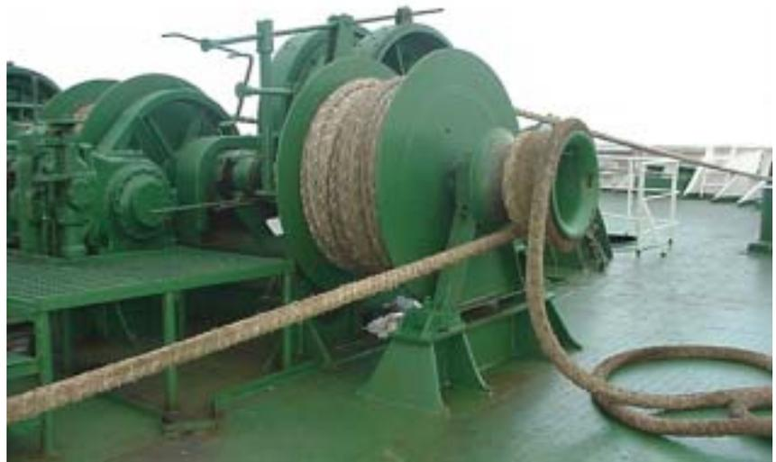
2. The drum ends are not designed for sustained, heavy loads, which can cause damage to the drive shafts, bearings and gearing mechanism.
