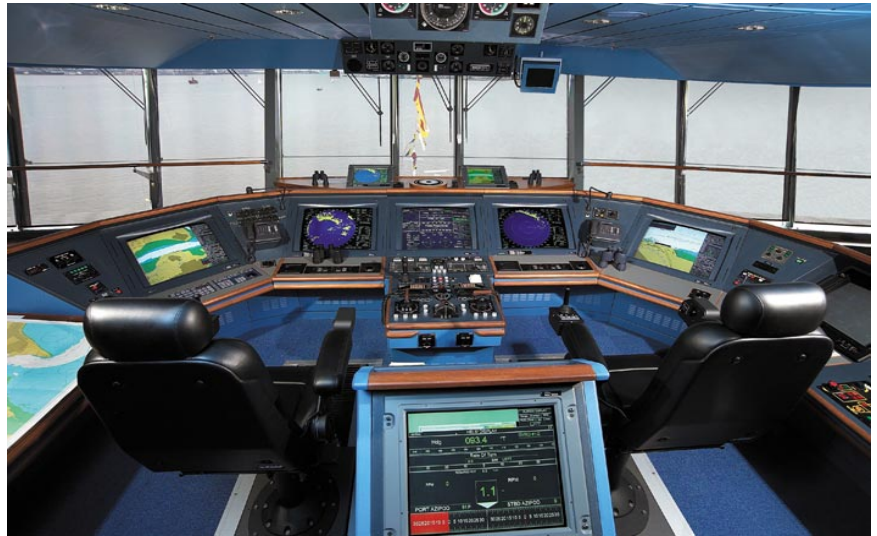
An integrated bridge system - Northrop Grumman Sperry Marine BV
